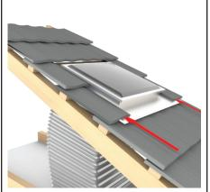
Slide the soaker tray up under the top and side tiles and over the bottom tiles.
