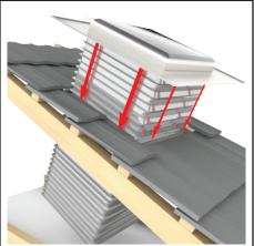
Gather up the flexi shaft, and gently lower the shaft through the opening in the roof, leaving it hanging inside the roof cavity.
