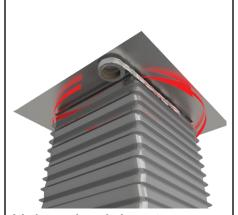
Using aluminium tape provided, secure flexi shaft to zincalume shroud at bottom of roof assembly.
