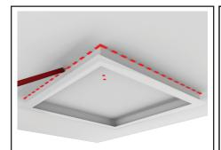
Back inside, using the direction holes as reference, place the inner ceiling frame corner against the corner hole.
