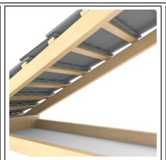
Decide location for skylight by inspecting inside roof cavity for obstructions such as hanging beams, under purlins, etc. Whenever possible, locate the ceiling ring directly below the roof assembly. Also, try to locate one edge of ceiling frame next to joist/truss.
