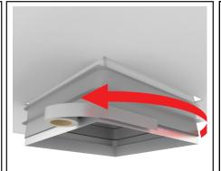
Slip flexi shaft over outside of zincalume shroud. Secure with a loop of tape provided.
