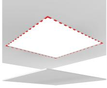
Using a plaster knife or jigsaw, cut along the marked line and remove the excess plaster.
