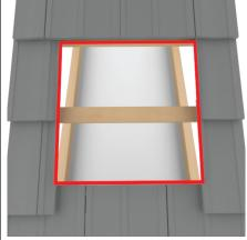
Place soaker tray in desired position and remove tiles. The lower edge of the skylight *opening* should be touching the top of the tiles on the low side.
