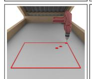
Drill a marker hole in ceiling to indicate one corner of the ceiling frame. Place two more holes to indicate direction of skylight.
