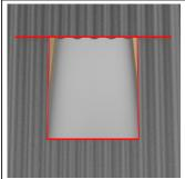
Using jigsaw or tinsnips, cut out marked lines and remove roof sheet piece.
