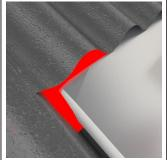
Backfill extended cuts at top corners of soaker tray with silicone.
