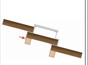
Space & attach brackets to Solar Panel so they align with the peak of Corrugations.
