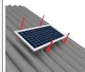
Attach brackets to the roof with screws. Seal under the screws. Run cable under ridge cap and into roof cavity.
