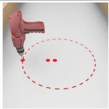
Using a drill, mark the edge of where the ceiling ring will be located in the ceiling.
