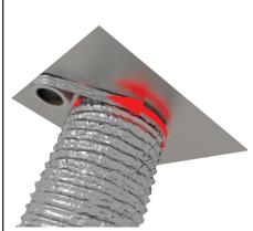
Fix the flexi shaft to the collar on the underside of the dome using the aluminium tape provided.
