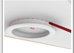
From ground level (looking up at ceiling) locate the original hole for positioning ceiling ring. Hold ceiling ring to ceiling with hole in dead centre. Trace the outside of the collar with a marker.
