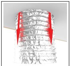
Pull excess flexi shaft through hole in ceiling.
