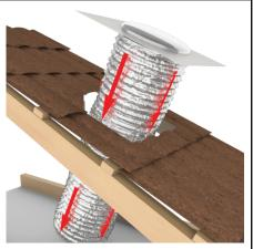
Drop flexi shaft through the opening in the roof sheeting.
