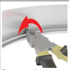
For non ventilated skylights: Using pliers, grip and twist white molded tabs inside ceiling ring to snap off.
